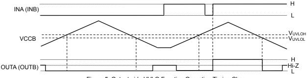
Figure 5. Output-side UVLO Function Operation Timing Char
