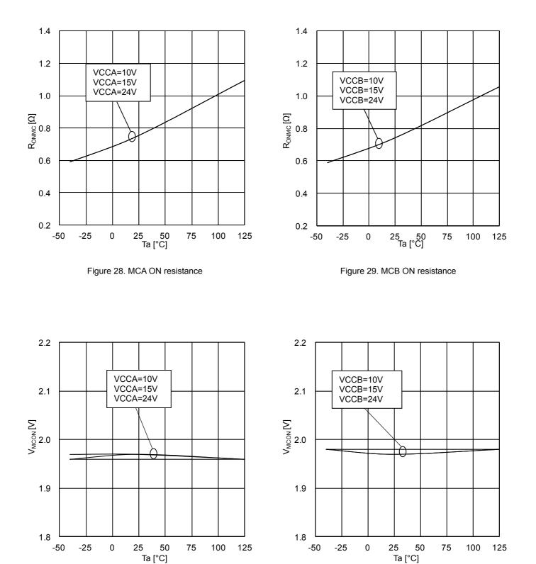
Figure 30. MCA ON threshold
